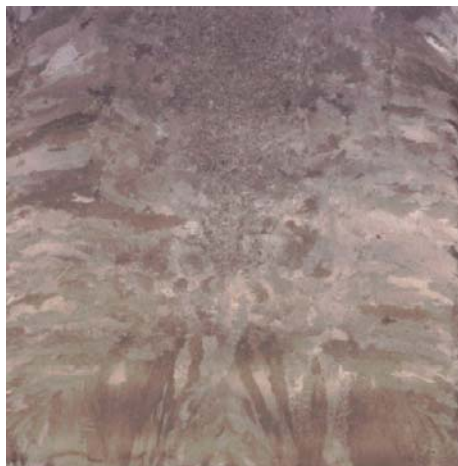
Fig. 1 Typical structure in a 200 mm cube used for property evaluation. This micrograph is XN50 TF
